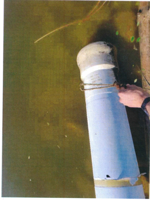
Figure 22: Safety buoy cable frayed through
